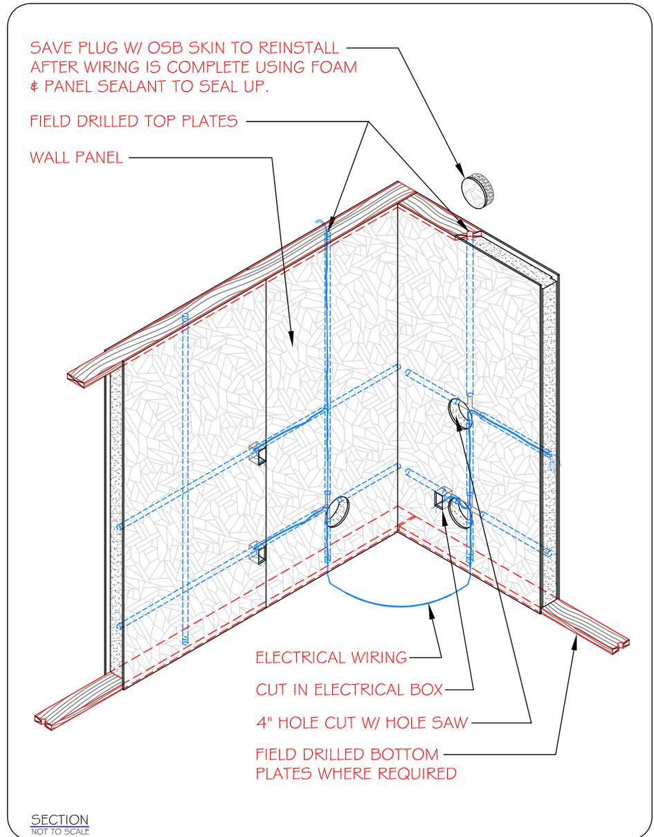
the default factory electrical chases are sufficient to provide adequate access for electrical runs; however, it would be best to review the SIP shop drawings<sup>1</sup> with your electrician and let your SIP manufacturer know if you would like to add any additional electrical chases within the SIPs.
