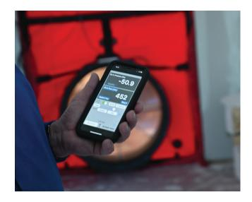
Be aware that blower door air leakage tests are also conducted by creating a pressure difference of 50 pascals between the inside and outside of the structure being tested. The leakage rate is often referred to as air changes per hour at 50 pascals of pressure or ACH50. Properly installed SIP structures regularly achieve leakage rates below 2.0 air changes per hour at a pressure of 50 pascals (ACH50), to as low as 0.3 ACH50 which is below the Passive House standard of 0.6 ACH50.
