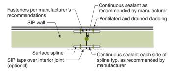
Details 1.1 through 1.7 depict different types of spline joints connecting panels (not to scale). As previously mentioned, solid lumber insulates less and transfers energy. Wood typically has an R-value of 1/inch compared to EPS foam at 3.6/inch minimum R-value as per ASTM C578 Type I foam. This is why the box/ block and surface splines are more thermally efficient than solid wood. A box/block and surface spline can be thought of as an 'insulating spline.'
