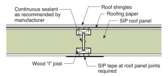
DETAIL 1.5: SIP ROOF - BOX/BLOCK SPLINE JOINT<sup>11</sup>
