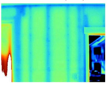
**IMAGE 1.6:** SIP GARAGE WITH LOW THERMAL **BRIDGING IN WALL/ROOF**
