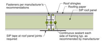
DETAIL 1.2: SIP ROOF - DIMENSIONAL LUMBER SINGLE SPLINE JOINT<sup>8</sup>
