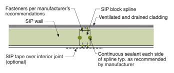
DETAIL 1.7: SIP WALL - SURFACE SPLINE JOINT<sup>13</sup>
