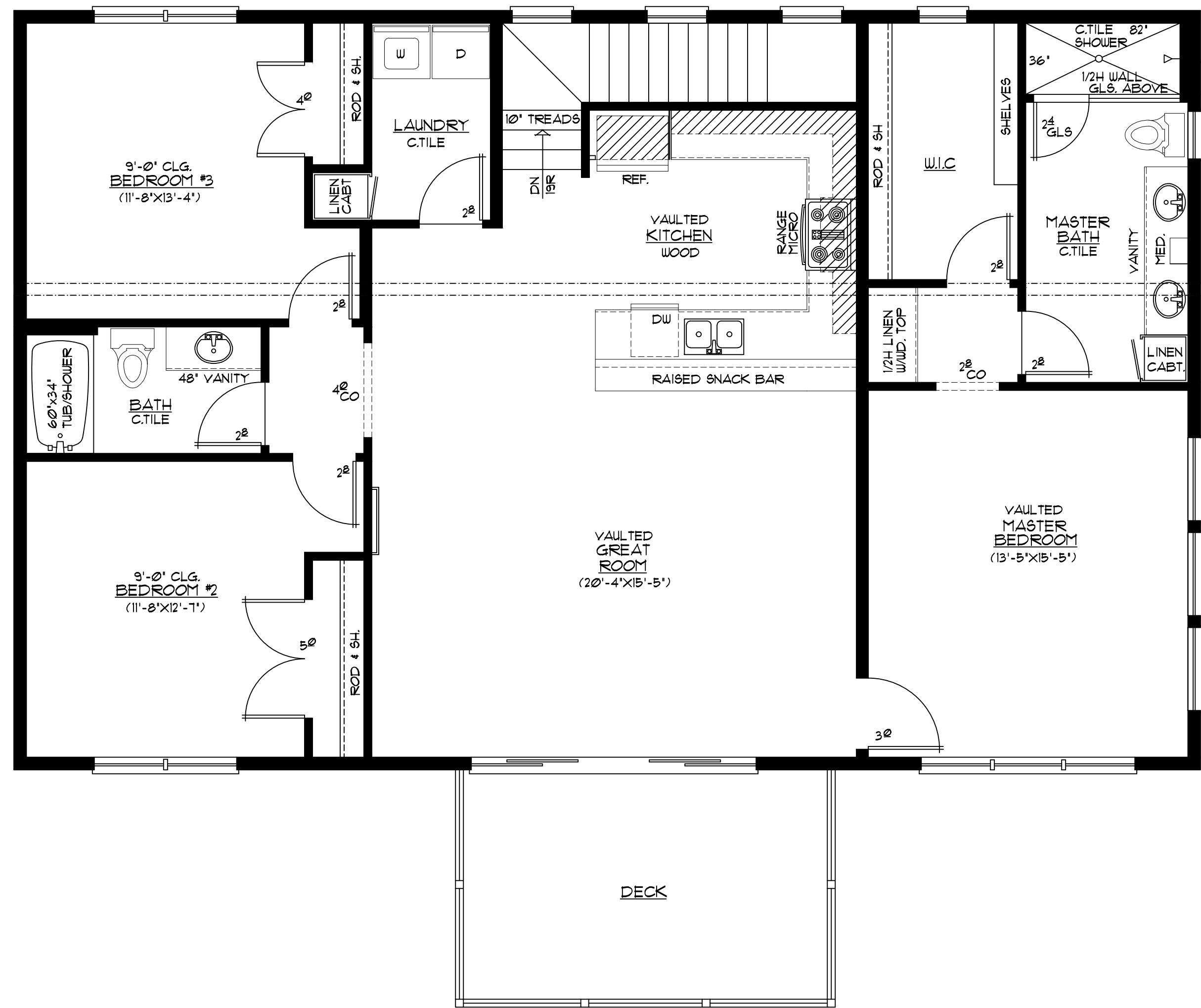
50'-0" x 32'-0" SECOND FLOOR PLAN 1/4" = 1'-0" 1600 SQ. FEET
