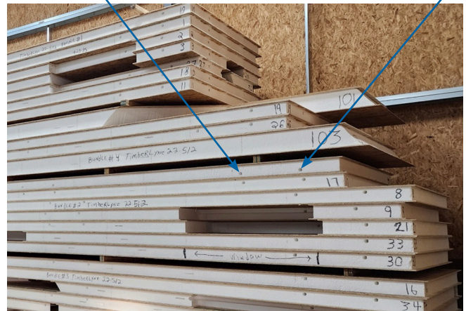
Horizontal chases at outlet height
