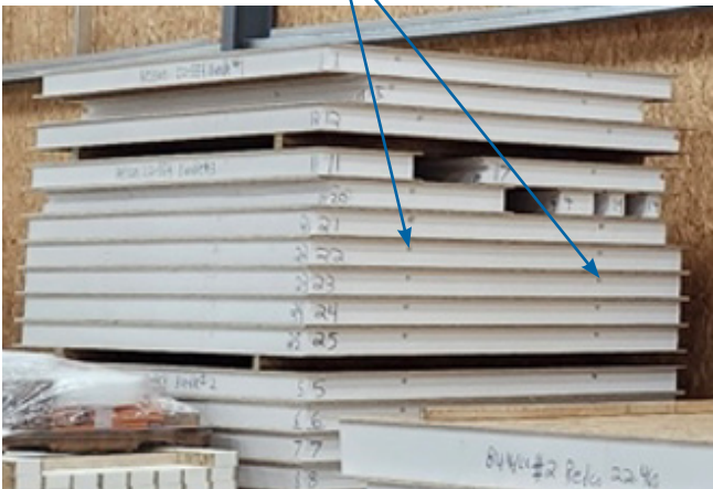
Horizontal chases at switch height
